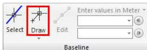
Using your left mouse button click on the two points along which you want to make the long section. The points are highlighted in the window and a corridor is created on the right and left sides.
