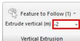
All the buildings will now be extruded from the roof heights, and 2 m under the ground surface, to simulate a cellar.
