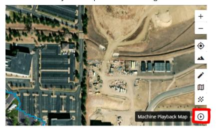
From within the tool, you can select a machine and a date/time range (currently limited to a 4 hour period). All production data from within the selected timeframe will be animated in the map view at a rate of roughly 1-2 seconds per minute of data, with the option to speed the animation up to 16x.
