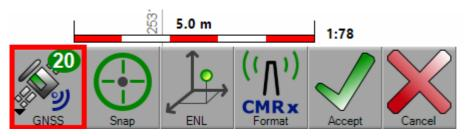
Snap a node for the base station position
