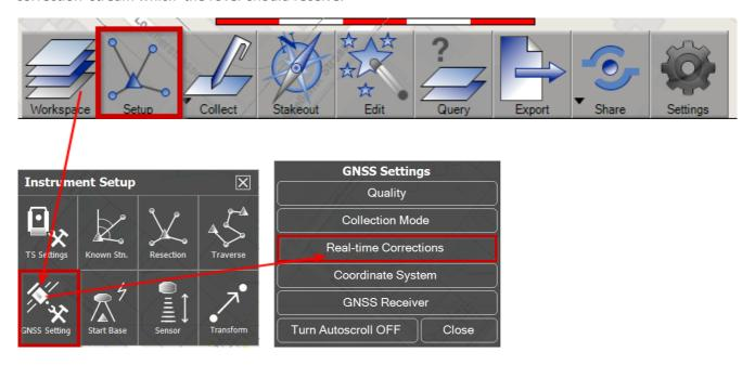
Set a new real-time correction service with **New**. Define the name of this service like **"Radio"**.
