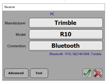
Open the real-time corrections via **Setup >> GNSS Settings >> Real-time Corrections.** This is the real-time correction stream which the rover should receive.
