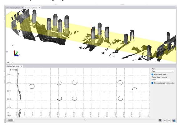
2. In Cutting plane view we would like to select all necessary scanned piles and with macro, we would like to create best-fit circles for all selected "piles".
