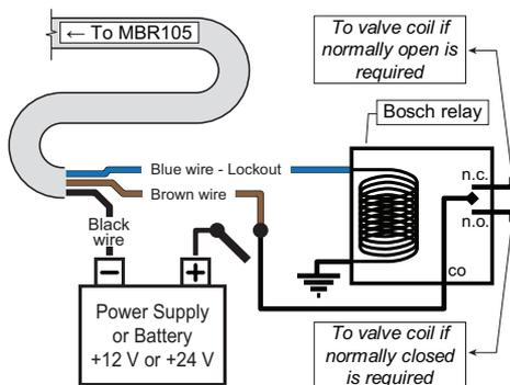
Connection with blue wire lockout and recommended Bosch relay.
